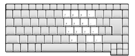
To use the the embedded numeric keys, toggle the Num Lock on by pressing the Fn + t keys simultaneously. With the embedded keypad turned on, the following actions are possible:
